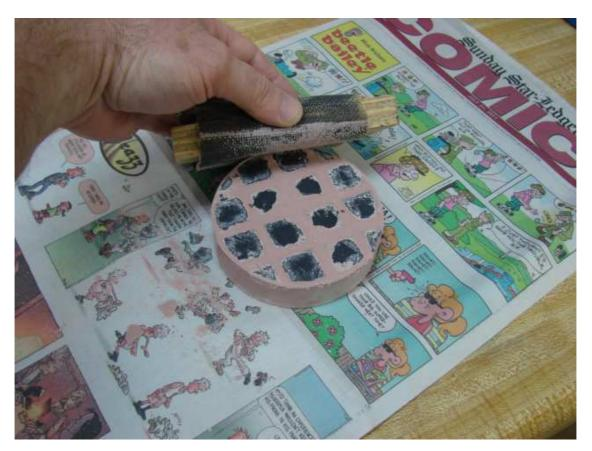
14. There may be a very thin film of plaster over some the tile faces, this will grind off in the first few grinding sessions. Let the tool dry/harden overnight.
