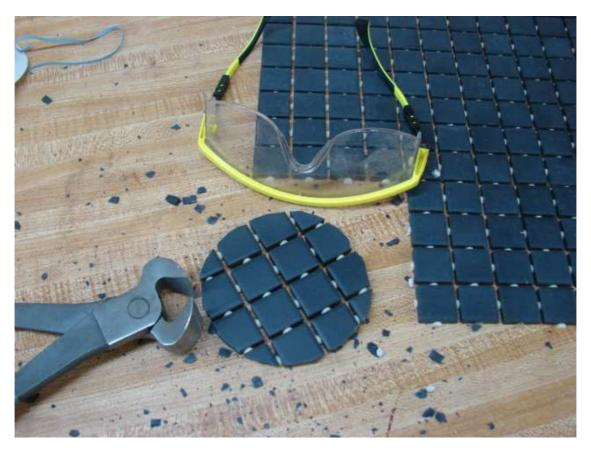
3. Make a form/dam that fits tightly around the outside of the blank. This can be made from a section of vertical blinds or a short length of aluminum flashing that goes around the circumference of the blank at least one and a half times. Use tape to keep the form from unrolling. The form should extend above the face of the blank at least the thickness of the blank.
