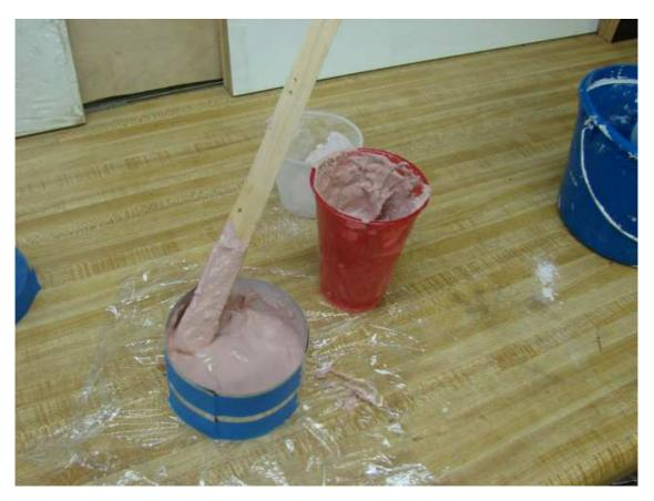
Pour more plaster to the desired thickness and smooth the top. Walk away for at least 20 minutes. Dental Plaster sets in less than 30 minutes. The surface of the plaster will begin to look dry and will be hard to the touch.
