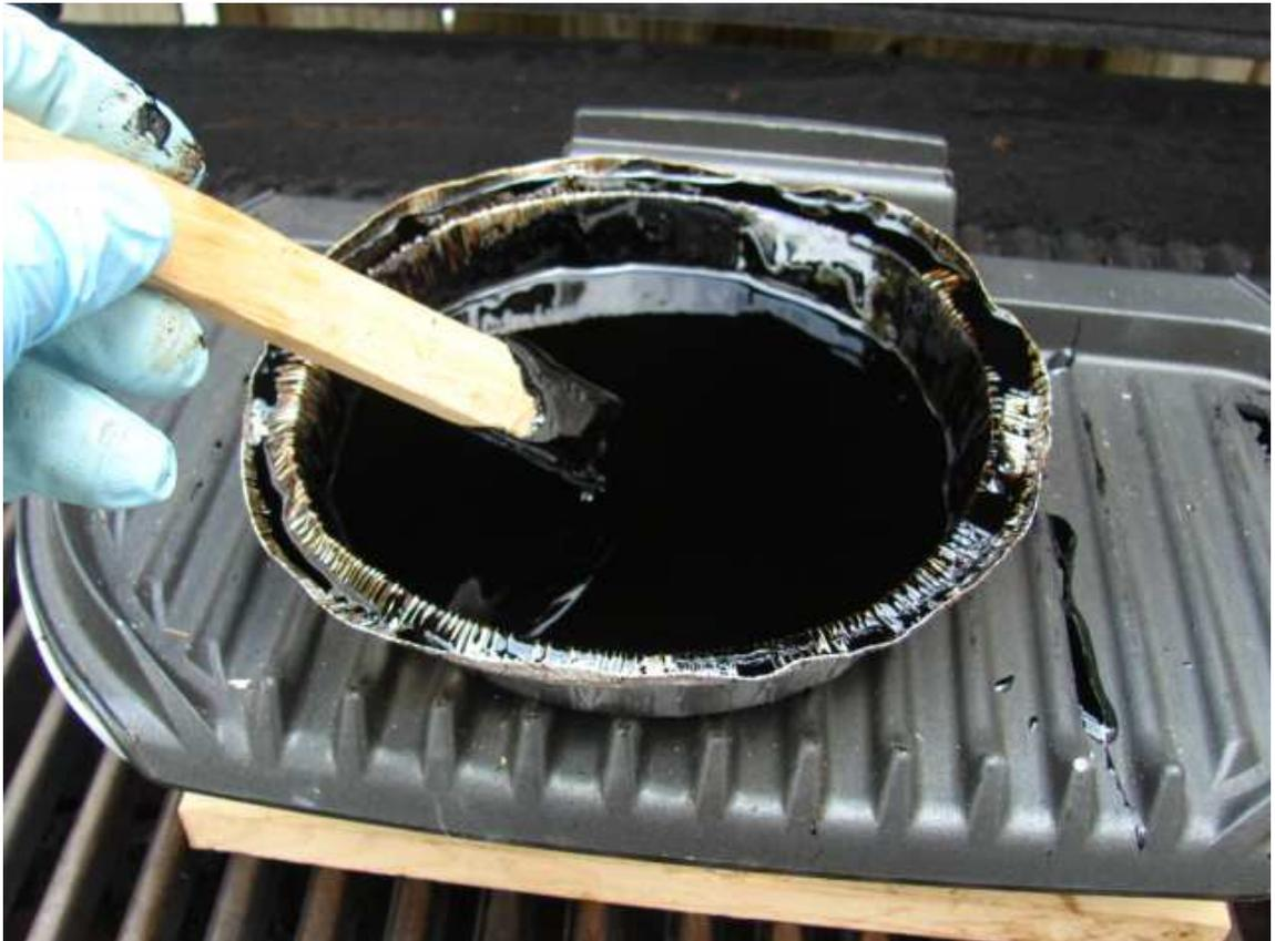
7. Once the pitch has completely melted and is a liquid, pour it onto the face of the backing piece. Pour onto the center. The pitch will flow to the edges quickly. You may get some bubbles. Don't try to fix them.
