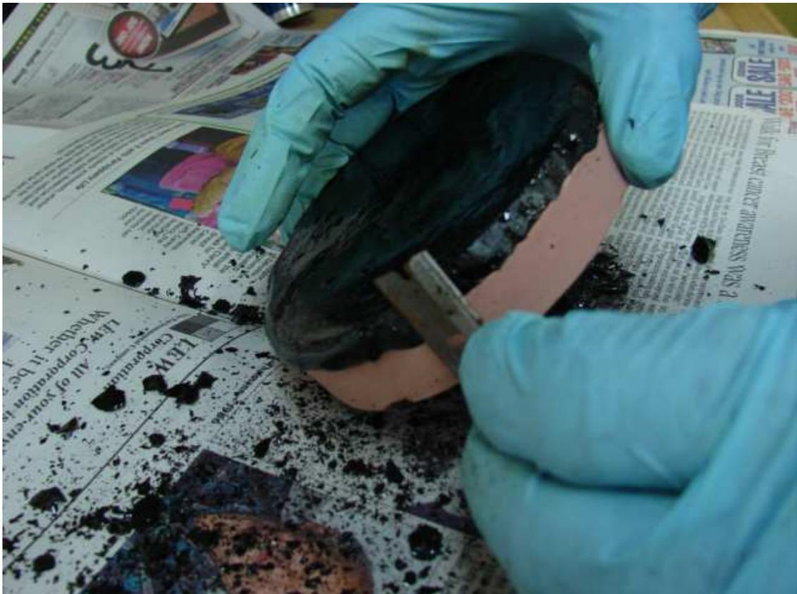
12. Next, cut facets into the laps. Use masking tape to mark where you will cut the facets at the tape's edge. Use a single-edge razor blade to scratch a "V" groove all the way across the lap. Try to make the first set of grooves about  $\frac{3}{4}$ " to 1" apart. Some mirror makers like to offset the first facet slightly off center. They believe a symmetric pattern of grooves is less likely to create a nice spherical polish and that a more random pattern is better.
