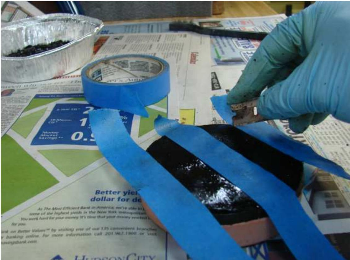
13. Use a BRASS wire brush to clean out the grooves between the facets as you cut them. Brass is better than a steel or stainless steel brush when working around glass. If a piece of the steel brush breaks off or becomes imbedded in the pitch, it will scratch the mirror next session. Brass will not. The grooves should be "V" shaped.
