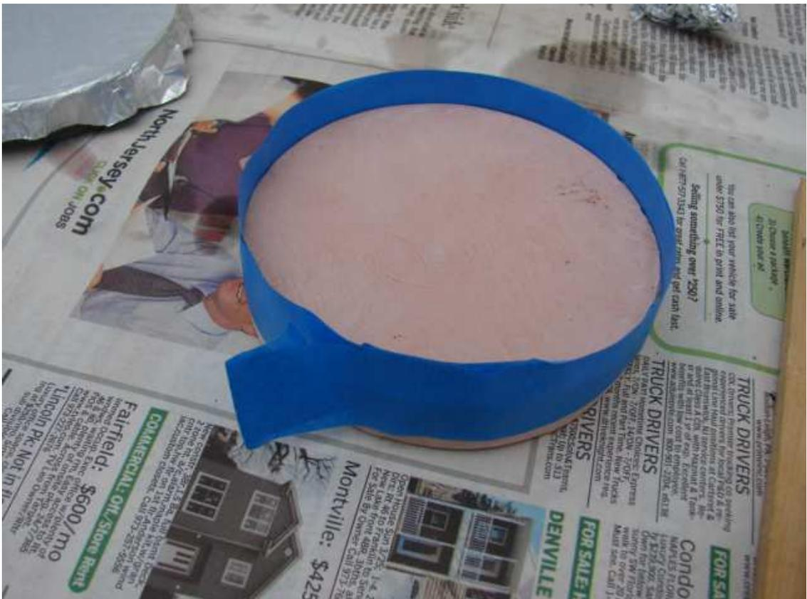
4. Rub a few drops of vegetable oil onto the mirror face. The oil helps to stick the foil to the glass. It also helps when you will be slipping the mirror off the foil in a later step.
