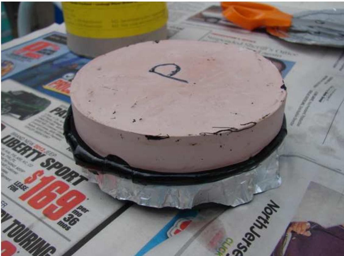
10. Once the pitch is somewhat hard, you can gently separate the mirror from the foil by sliding it **SIDEWAYS** and off the edge. If you try to pull or pry them apart you will make a dent in the pitch, or worse, pull the soft pitch off the backer. Here is a photo showing the lap after the mirror has been removed and the aluminum foil peeled off too.
