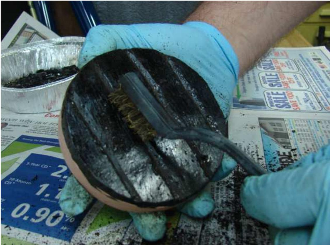
14. Cut more grooves at right angles to the first set. A “waffle” pattern results. Brush again, and you are ready for pressing before polishing.
