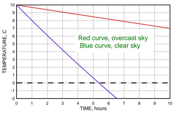
**Figure 2. Night Radiation Loss Temperature Profiles**
