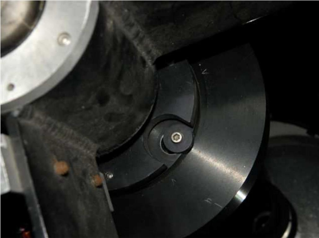
**Photo 7** This photo illustrates how far the secondary needed to be shifted laterally to center it
