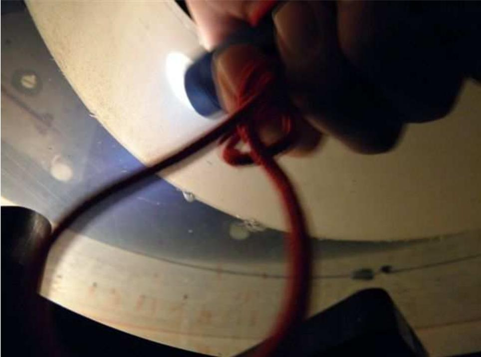
**Photo 6 Illuminating the backside of the mirror to check for pinholing of the coating**
